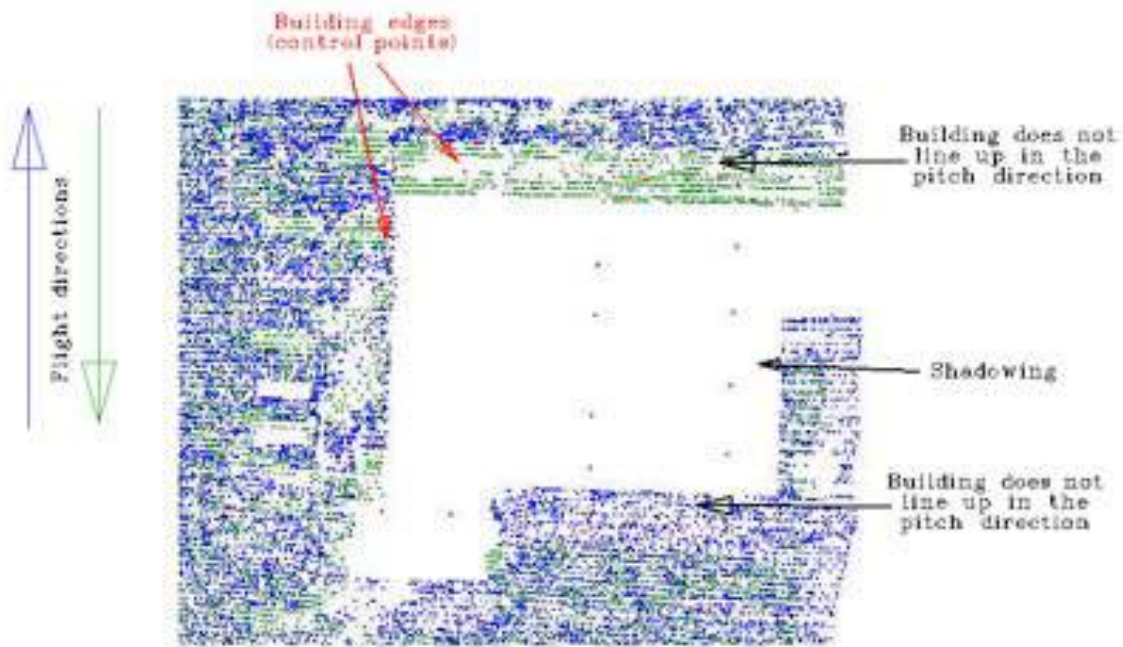
8 – Top view of two laser swaths with a one-degree pitch offset error.
